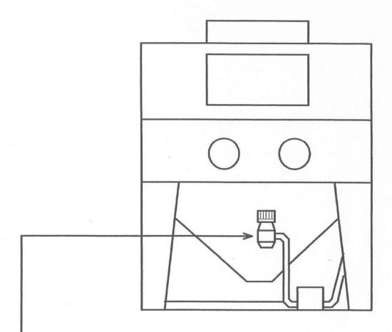
Blast cabinet must be supplied with compressed air delivered through a minimum of 1/2" I.D. air hose or piping. Distances greater than 25 feet require 3/4" I.D. Air inlet is 3/8" female thread. \* Standard size supplied unless ordered otherwise.
